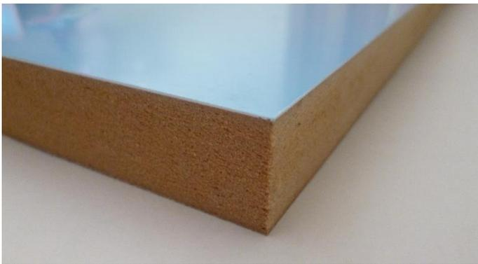
The MDF panels used for the production of the furniture units have a thin veneer of PVC for colour and protection.
