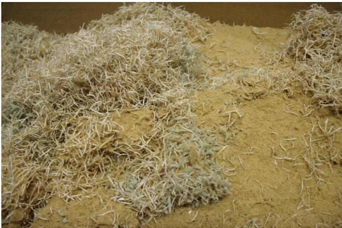
In its ex-works state, the material is an MDF-heavy mix of MDF dust and thin PVC turnings. Compositional analysis shows that the MDF accounts for around 83% of the weight.
