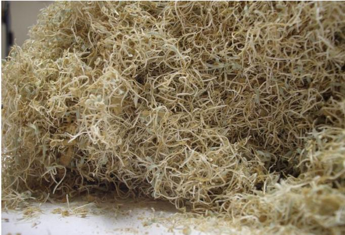
This image shows the sieved PVC material, which inevitably still has a small degree of MDF contamination.
