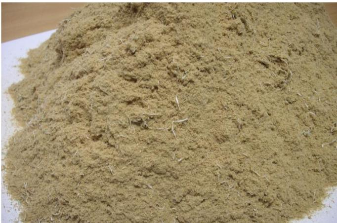
Separation of the two fractions is possible with a suitable sieve. The dust in the image here was screened using a standard kitchen sieve and it can be seen that some PVC managed to get through, though this can be resolved by double-sieving or by using a finer grade of mesh.
